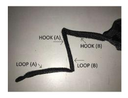
This is a diagram indicating how the HOOK and LOOP parts are sewn to the strap.
